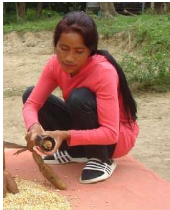
Fig. 2. Maize shelling using Octagonal Hand Maize Sheller
